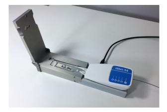
The InterMet Ground Check Unit is used to quickly and easily confirm correct operation of iMet-54 radiosonde sensors before use. The unit uses very stable humidity and temperature reference sensors to ensure consistency and accuracy from all iMet-54 soundings.
